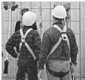
BODY HARNESS Max. Arresting Force = 1800 lbs.
